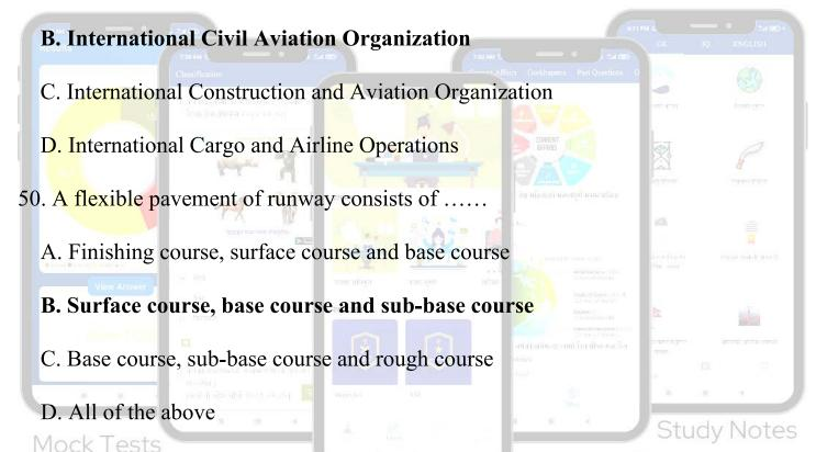
A flexible pavement of a runway typically consists of the **surface course**, **base course**, and **sub-base course**. These layers work together to distribute loads, resist deformation, and provide durability. The surface course is the topmost layer made of asphalt, the base course provides structural support, and the sub-base course further distributes loads to the subgrade beneath
